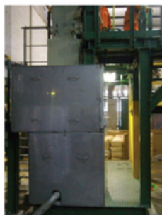
After: Same shredder machine fully covered up with removeable noise reducing panels.
