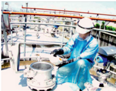
Before: Manual pouring of acid into storage tank
