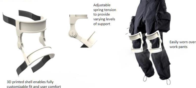
Figure 31: Example of a design concept for a wearable device that can provide knee extension assistance for workers who spend long hours walking/climbing
